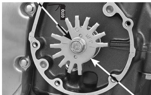
ROTOR DO SENSOR CKP SENSOR CKP
